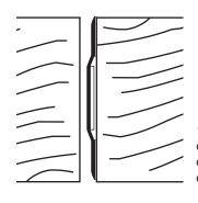
1/8" clearance required between doors and between door and frame
