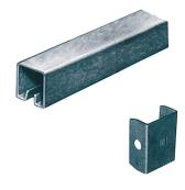
**No. 5116 Rail**—For doors weighing up to 450 lbs. per panel. 16 gauge galvanized steel rail bundled without fasteners or brackets. Can be used with various types of single and multiple brackets.
