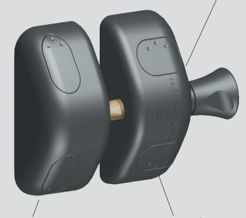
The MagnaLatch Side Pull model allows for easy horizontal and vertical adjustment with just a turn of a screwdriver. It can be adjusted up to 3/8" (10mm) at any time during or after installation. This feature compensates for ground settling and gate movement that may occur over time. The adjustability of MagnaLatch ensures the gate will continue to operate properly long after installation.
