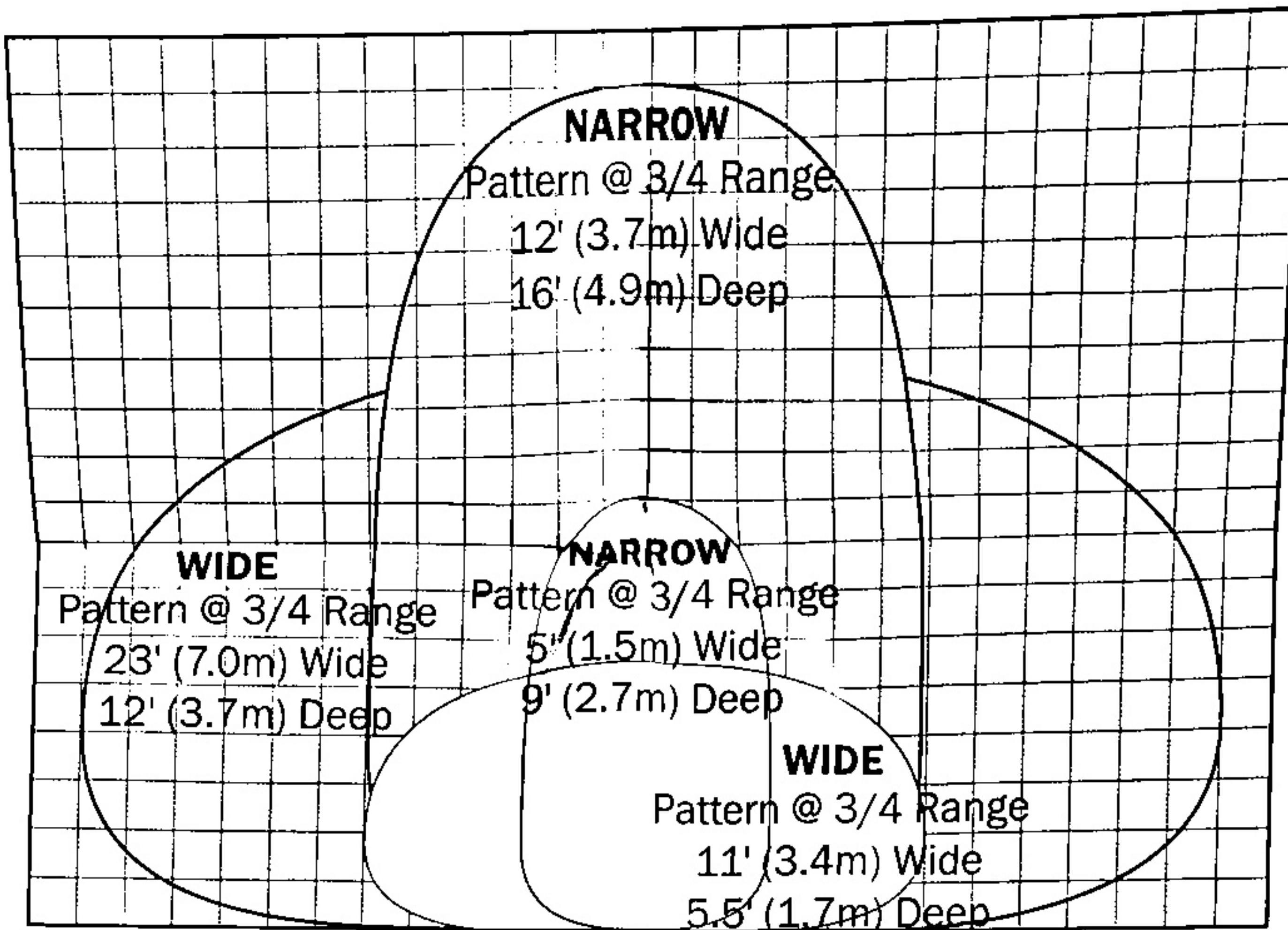
NOTE. The smaller detection patterns shown are from a D38 mounted 7'6" above the finished floor with an elevation angle of 27°. The larger detection patterns shown are from a D38 mounted 15' above the finished floor with an elevation angle of 27°. All patterns shown are approximate and can vary slightly. Walk test the unit to assure the pattern desired.
