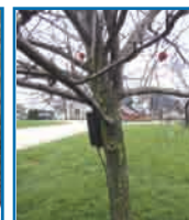
DA-611TO sensor buried by the drive, transmitter hidden in a tree
