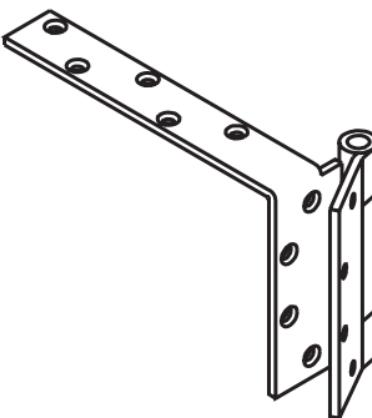
Anchor plate for door header only. Permits use of holders, closers concealed in top of jamb.
