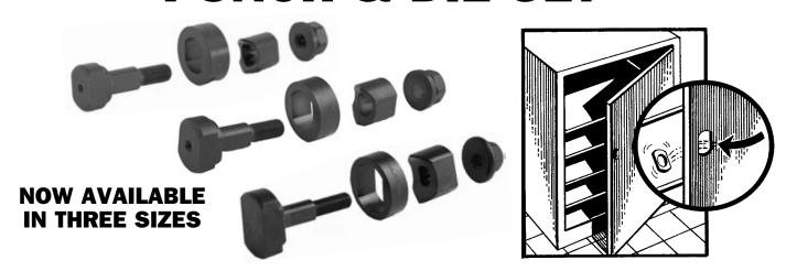
Major Manufacturing's punch and die set will punch a **DOUBLE "D"** hole in sheet metal cabinet drawers and doors. A must have tool for the locksmith working on vending machines, lockers, metal cabinets or any type of sheet metal door made with 18 guage (.048) or lighter steel. To use, simply drill a 1/2" hole centered where the cam lock is to be installed, slide the punch through the hole and tighten down the hex nut with a 11/16" wrench or socket set.
