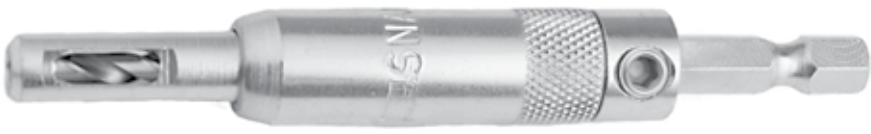
Use our self centering drill guides when drilling pilot holes for mounting screws used in mortise lock bodies, latch faces, hinges, etc. Because the hole in the hardware is larger than the drill bit used to make the pilot hole for the screw, it is hard to drill the hole in the exact center. An off center pilot hole can cause mis-aligned hardware and possible binding or crooked looking installation.
