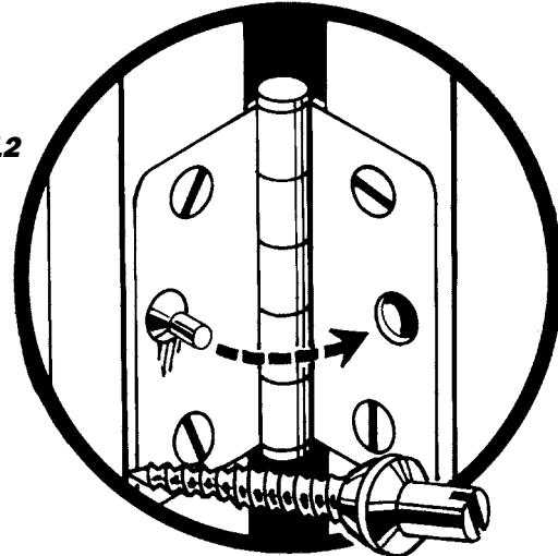
■ **JP-10 & JP-12 Pins:** Simply remove one opposing screw from each hinge leaf and replace with the proper size Jamb Pin.
