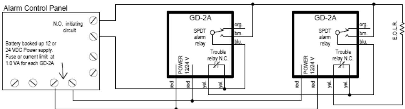
6. The GD-2A uses a full wave bridge rectifier at its power input, so that it is independent of the polarity of the input power. It can operate on DC or AC voltages between 12 and 24 volts.
