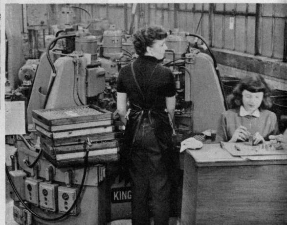
Seven station, fully automatic machine for precision drilling and tapping operations.
