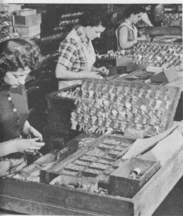
Pin tumbler cylinder assembly.
