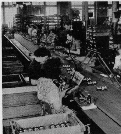
Belt assembly line, cylindrical lock sets.
