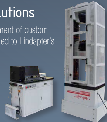
(Above) One of two 224,800lbs testing machines in Lindapter's Research & Development Facility
