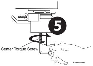
Slowly Rotate Center Torque Screw clockwise until you feel the assembly loosen.
