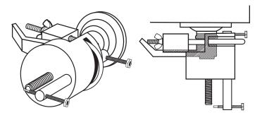
Lever Handle Remover aligned on lever.
