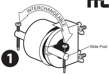
Determine the proper size Pin Depressing Screw and place on operational end of slide post.
