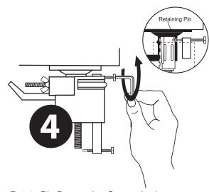
Rotate Pin Depressing Screw slowly just enough to enter inside of lever wall and hold retaining pin in.
