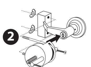
Remove Vice-Block and Wing Nuts. Mount assembly to Lever as shown. Re-attach Wing Nuts and align to lever. Do not tighten Wing Nuts.
