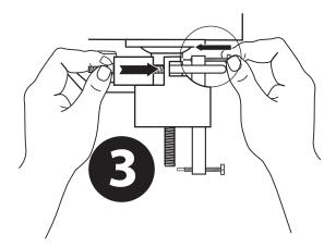
Line up Pin Depressing Screw and tighten Wing Nuts.
