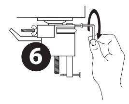
Loosen Pin Depressing Screw away from wall of Lever.
