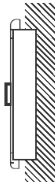
2\frac{1}{2} ", 3\frac{1}{2} ", 4 " or 4\frac{1}{2} " Rolled Edge Semi-Recessed
