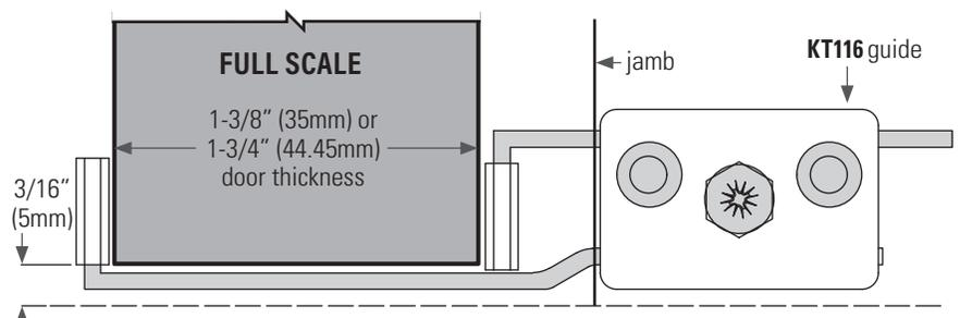
**KT116** Adjustable bottom guide (metal & plastic), for doors up to 1-3/4" (45mm) thick
