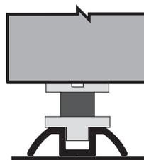
**KT114** Bottom guide (plastic), spring loaded, for KT19 floor channel
