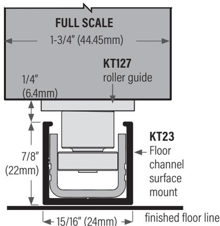
**KT127SS** Bottom guide, ball bearing roller (stainless steel) for surface mount floor channel
