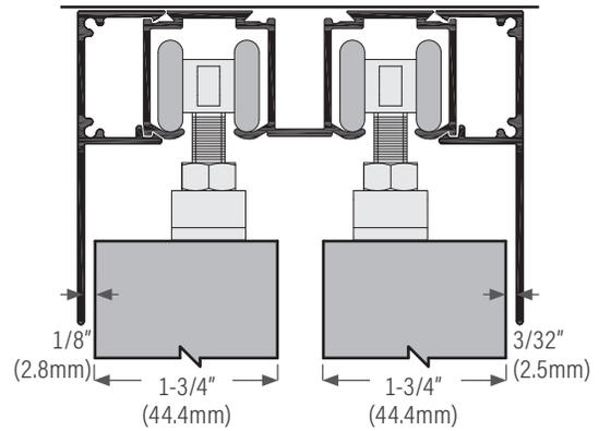
for room divider application track is installed wall to wall, no open end of track showing
