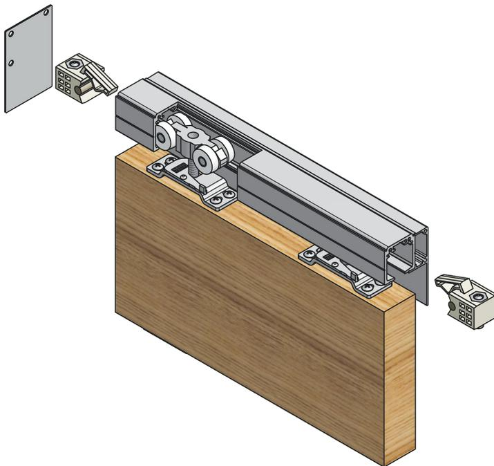
**2X SINGLE TRACK FOR BYPASS APPLICATION. FASCIAS BOTH SIDES FOR ROOM DIVIDER APPLICATION.**
