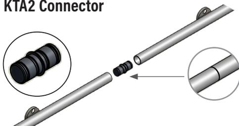
**NOTE:** For biparting double doors, 2 kits required plus one connector piece (KTA2RAILCON)
