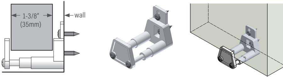
**KT113** Adjustable bottom guide for wall face mounted door for 1-3/8" or 1-3/4" door thickness
