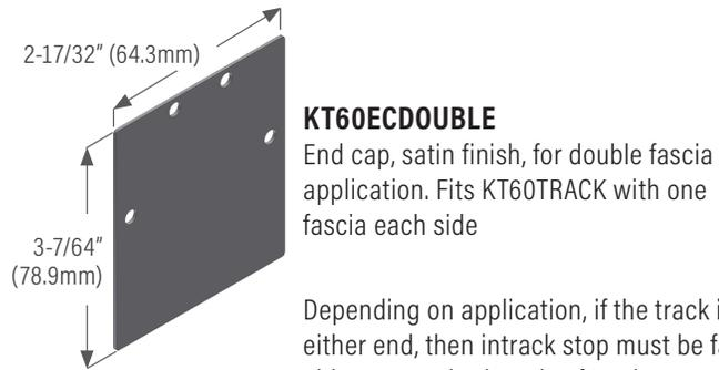
Depending on application, if the track is open at either end, then intrack stop must be fastened to either one or both ends of track.
