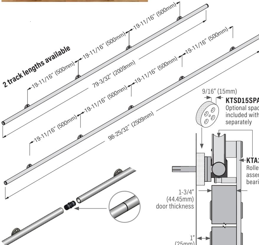
**KTA2RAILCON** Connector piece, connects 2 pieces of rail end to end. Order separately.
