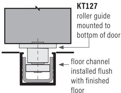
**KT23DV** Floor channel bronze anodized with PVC insert. Lengths available: 36\", 72\", 111\", 147\", 183\", 222\", 294\" (914mm, 1829mm, 2819mm, 3734mm, 4648mm, 5639mm, 7468mm)
