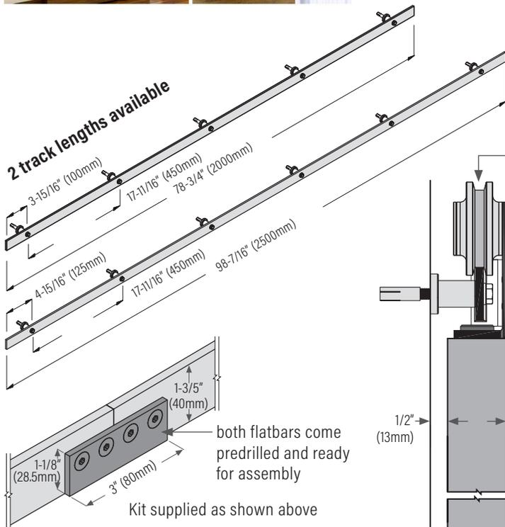
Connector piece, connects 2 pieces of flat bar end to end to extend length for biparting doors.
