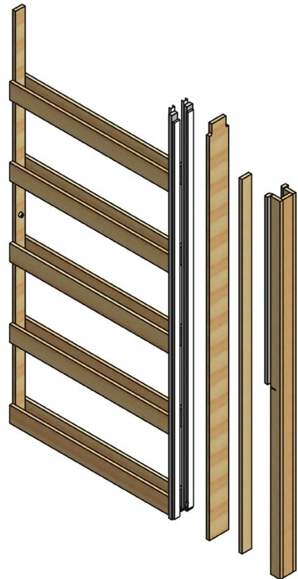
**NOTE:** replace all track screws with # 8 x 1-1/2" (38mm) screws (included) after frame is installed and before drywall.
