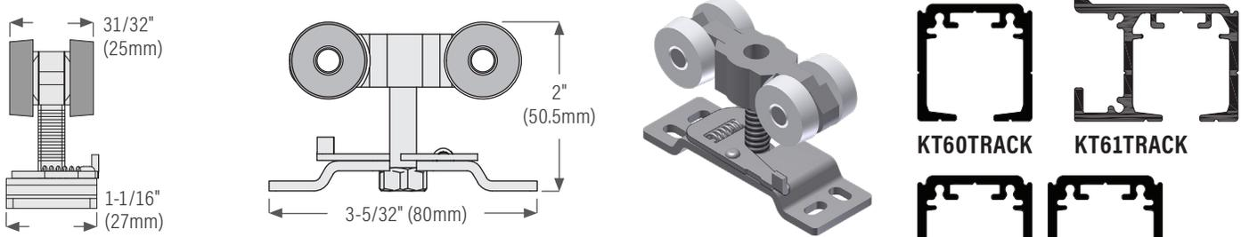
**KT60HANGER** for KT60 & KT61 sliding door track. Max door weight: 132 lbs (60 kg) = 2 hangers
