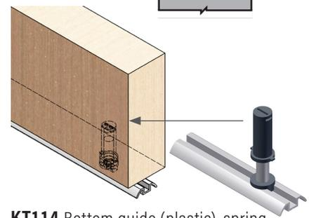
**KT114** Bottom guide (plastic), spring loaded, for KT19 floor channel
