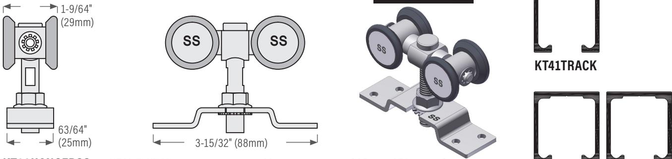
**KT82HANGERSS** for KT41 & KT51 sliding door track. Max door weight: 385 lbs (175 kg) = 2 hangers
