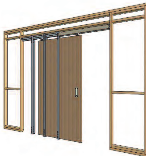
2 X 6 WALL CONSTRUCTION POCKET DOOR KIT SECTION VIEW
