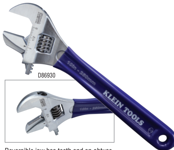
Reversible jaw has teeth and an obtuse angle to work as a pipe wrench
