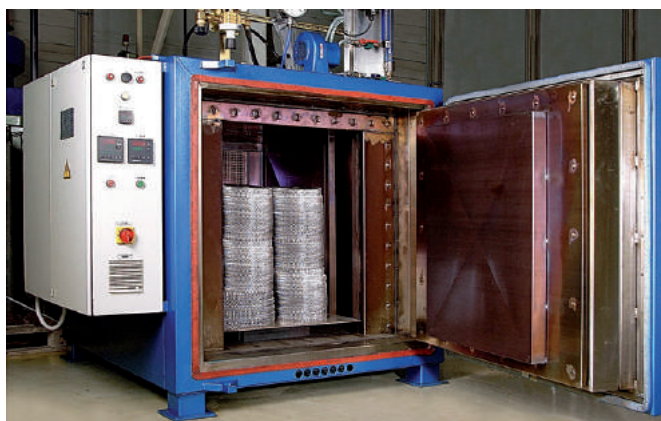
Anlassofen · Tempering Furnace
