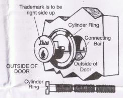
3. Place Backplate over connecting bar and attach to cylinder using two (2) break-off screws provided which are for 2¼" (57mm) doors; for thinner doors screws should be cut to proper length, depending on thickness of door (screws are provided with break-off points). IMPORTANT: Line up backplate ½" (3mm) from edge of door (see sketch above). Break off connecting bar so that it extends ½" (13mm) max. beyond face of backplate. Connecting bar is provided with break-off points.
