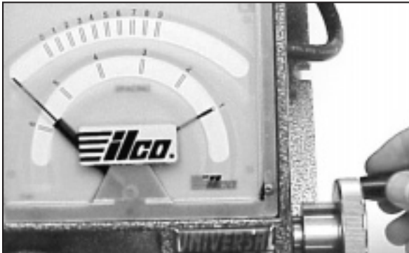
Rotating Spacing Crank to center Spacing Needle over desired cut position
