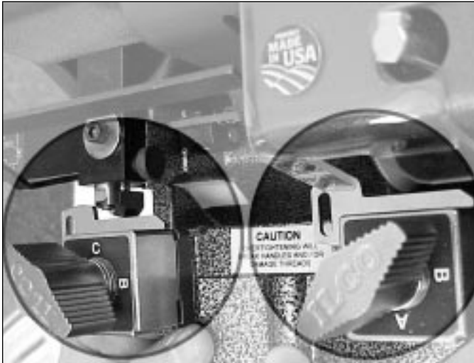
Figure 16 - Adjustment is correct when both keys touch
