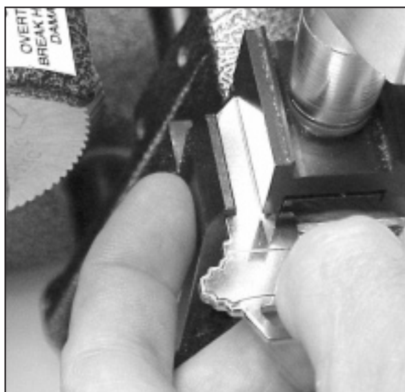
Shoulder of key is in contact with edge of gauge.
