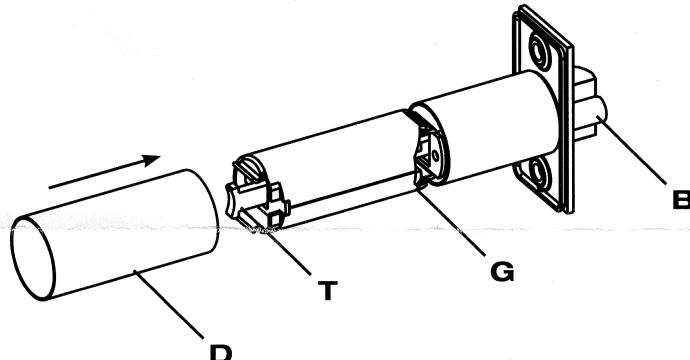
Fig. 3 Assemble sleeve "D" to hold both latch and latch extension.
