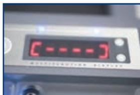
**2** Has an electronic regulation system that indicates the exact machine regulation point. The display shows the rotation direction of the adjustment wheel.
