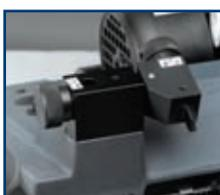
2 Tracer point with micrometric adjustment.
