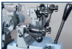
3 Blocking of slides on X and Y axis.
