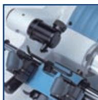
2 Tracer point with micrometric adjustment.
