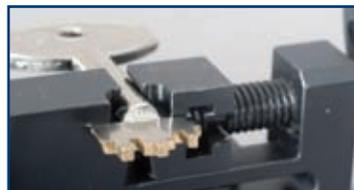
8 Milled clamps to correctly secure keys.
