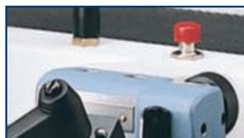
**2** Tracer point with micrometric adjustment.
