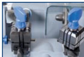
**3** New clamp turning system. Compatible with earlier key-cutting machines (Dakota, Titan, Saratoga...).
