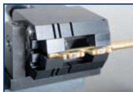
4 Clamps with adjustable jaws to correctly secure bit keys of different lengths.
