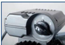
2 2-speed motor for brass and steel keys.
