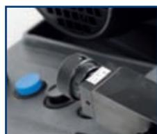
2 Tracer point with micrometric adjustment.
