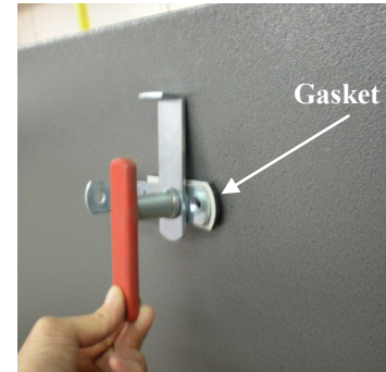
Rotate Red Handle on Exterior Handle so that Holes are Exposed
