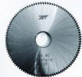
CUTTER NUMBER: 26MC STYLE: MILLING CUTTER DIAMETER: 3 1/8" - 80MM THICKNESS: .196" - 5MM HOLE DIAMETER: .630" MAT: M35 HIGH SPEED STEEL USE ON: JET 7060
