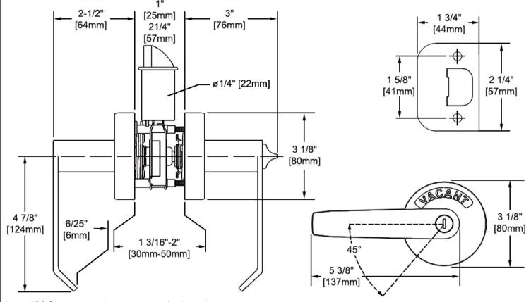
**Door Thickness:** Standard Doors 1-3/16" to 2" **Back set** -Standard is 2 3/8, 2 3/4" Adjustable
