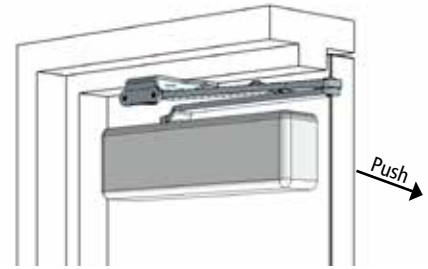
Parallel Arm (Push Side) Permits 180° maximum opening
