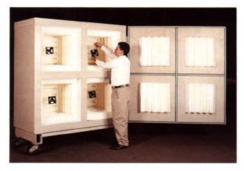
Multi-Compartment Mini-Anechoic Rooms are designed for testing a number of components simultaneously; quality control of components produced in quantity is one example.
