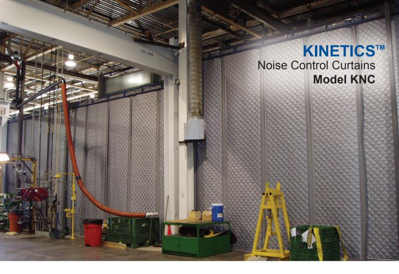
KINETICS™ KNC Noise Control Curtains are modular, reinforced limp-mass and quilted fiber-glass composites designed to block noise or to act as a movable barrier between noisy and quiet areas. Kinetics Noise Control Curtain Systems incorporate a self-supporting track which allows the curtain to open for access at virtually any point along the barrier or enclosure.
