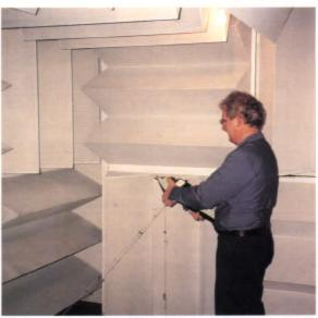
Fig. 4 – Prototype hemi-anechoic room fully treated with Metadyne Wedges at IAC Aero-Acoustic Laboratory in New York. Inside clear dimensions: 8 ft-2 in. x 12 ft-2 in. x 6 ft-10 in. high (2489 x 3708 x 2083mm).
