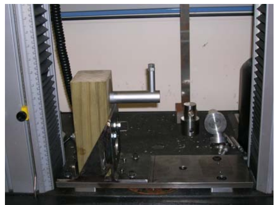
Fig 1 Jig used to apply compression loading to a HB 520 bracket assembly.
