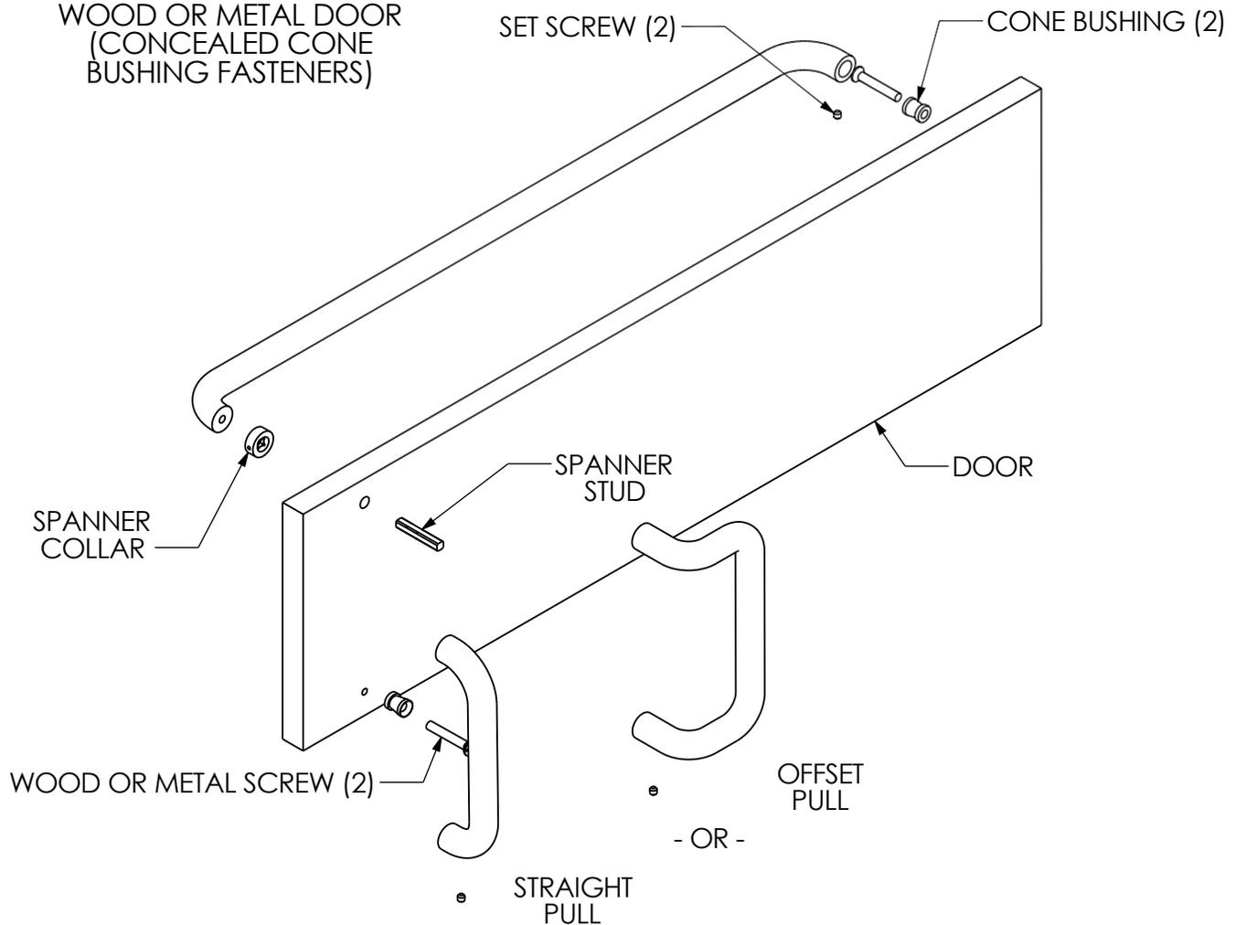
**NOTES: DO NOT FULLY TIGHTEN HARDWARE UNTIL SET IS COMPLETELY ASSEMBLED ON DOOR. RIV-NUTS, SUPPLIED BY OTHERS, ARE REQUIRED FOR INSTALLATION ON ALUMINUM DOORS.**
