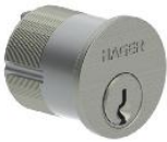
3902 Mortise Cylinder • Conventional cylinder supplied drilled 6-pin, keyed 5-pin standard • 3975 standard cam attached and 3972 Adams Rite cam shipped loose in the box • Thread size is 1.150" x 32 UNS • Cylinder face diameter is 1.360" • Supplied with two operating keys • 1-1/8" (29 mm) standard length, 1-1/4" (31 mm), and 1-5/8" (41 mm) for mortise exit devices • Other lengths may be available with extended lead time • Must specify length, cam, keyway, and keying requirements
