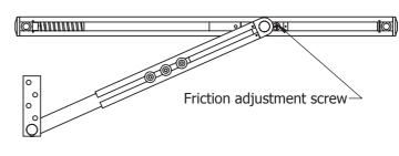
Using a flat head screwdriver, turn the friction adjustment screw clockwise to increase the friction and counterclockwise to lower the friction.
