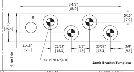
Cut out and tape parallel to the frame at the "B" measurement from step 2.
