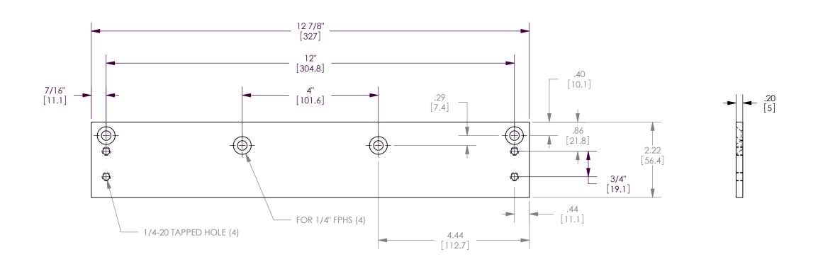
SCREW PACK INCLUDES: 4PCS. 1/4-14 X 1-1/2" FPHS SELF DRILLING (STEEL) 4PCS. 1/4-20 X 1-1/2" FPHS SELF DRILLING (STEEL) 4PCS. 1/4-20 X 7/16" FPHS (STEEL)
