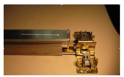
3. Set the push bar upside down on the table and remove the two screws that hold the dogging mechanism in place. Thread locker was used on these screws when they were originally applied. Be sure to press down firmly upon the screws or use an impact driver while unscrewing them in order to prevent stripping the heads.
