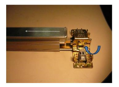
6. Reattach the push bar to the cover tube by installing the two screws.
