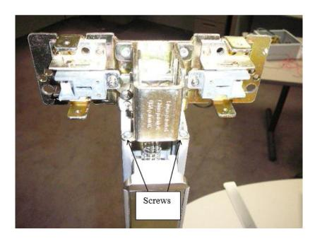
2. Slide the push bar out of the tube.
