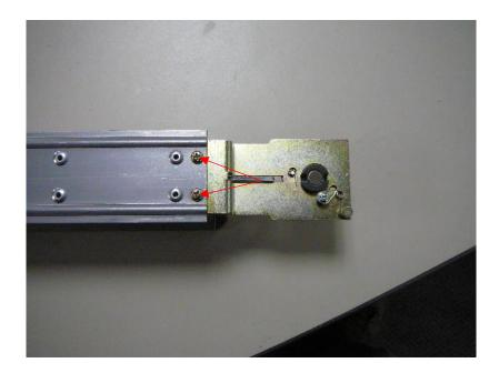
4. Attach the new dogging mechanism with the same screws.
