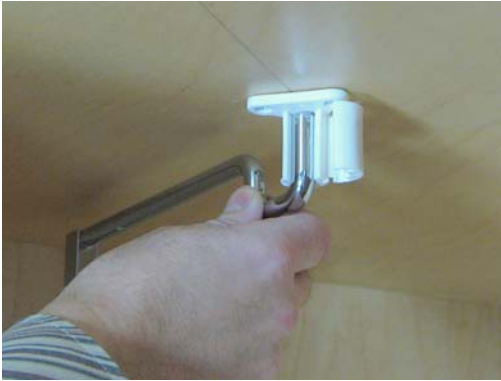
1. Put in the upper angle in the bearing
