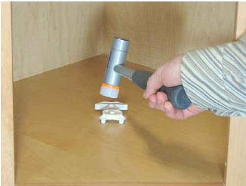
4. Put in bottom bearing
