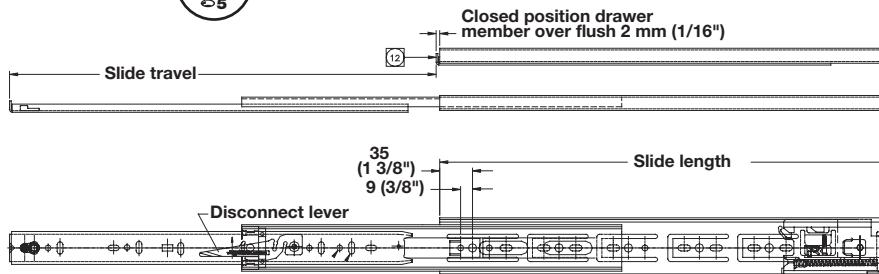
For optimal performance, construct drawer 27 mm (1 1/16") less than cabinet opening.
