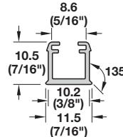
Routing dimensions W x D: 11 x 11 mm (7/16" x 7/16")
