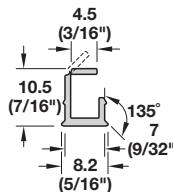
Routing dimensions W x D: 8 x 11 mm (5/16" x 7/16")
