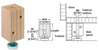
> Material: Steel; Finish: zinc-plated; Mounting block: Wood Cap: Plastic; Color: white
