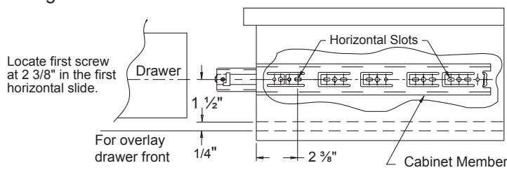
**Figure 2** 32 mm Mounting—Cabinet
