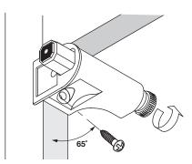
**Important:** Use a 65° angle for best mounting results. Pilot drill  $\varnothing 2.3$  mm (3/32") and 1/4" deep for a #6 x 3/4". Mount in upper corner on hinge side.
