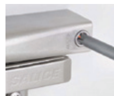
Rotate the screw toward the plus sign to decrease closing speed, or to the minus sign to increase closing speed
