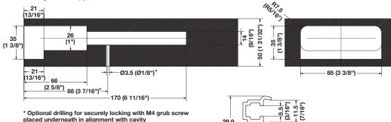
\* Optional drilling for securely locking with M4 grub screw placed underneath in alignment with cavity For details see Triade Maxi drawing
