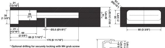
\* Optional drilling for securely locking with M4 grub screw placed underneath in alignment with cavity For details see Triade Maxi drawing
