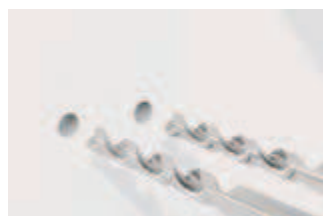
Drill Ø 8 mm hole for connecting bolt
