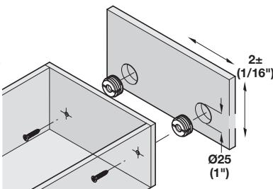
> One part drawer front adjusting fitting fits into a Ø25 mm (1") hole in the drawer front
