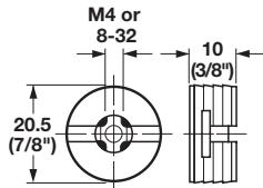
> Pressed in a 20 mm (3/16") hole in drawer front
