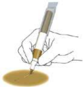
Step 1 Using marker tip, completely color in areas of scratch
