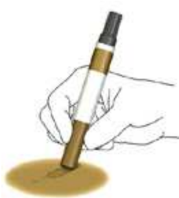
Step 2 Using wax stick, rub in fill material until scratch is filled
