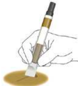
Step 3 Using leveler, skim off excess fill material until wax is completely removed and scratch fill is flush
