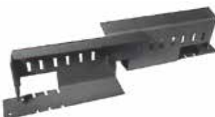
HEAVY DUTY ADJUSTABLE DRYWALL ANCHOR • 18 GA., fits frame sizes 5 3/4" to 8 3/4". • Anchors stamped with frame sizes for fast installation. • 2 pieces per set. • Ideal solution for anchoring larger size frames. 200 PCS (100 SETS) PER BOX
