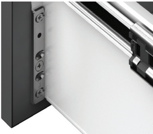
Adjustment via integrated front fixing bracket Height adjustment \pm 2\text{mm} Side adjustment \pm 1.5\text{mm}
