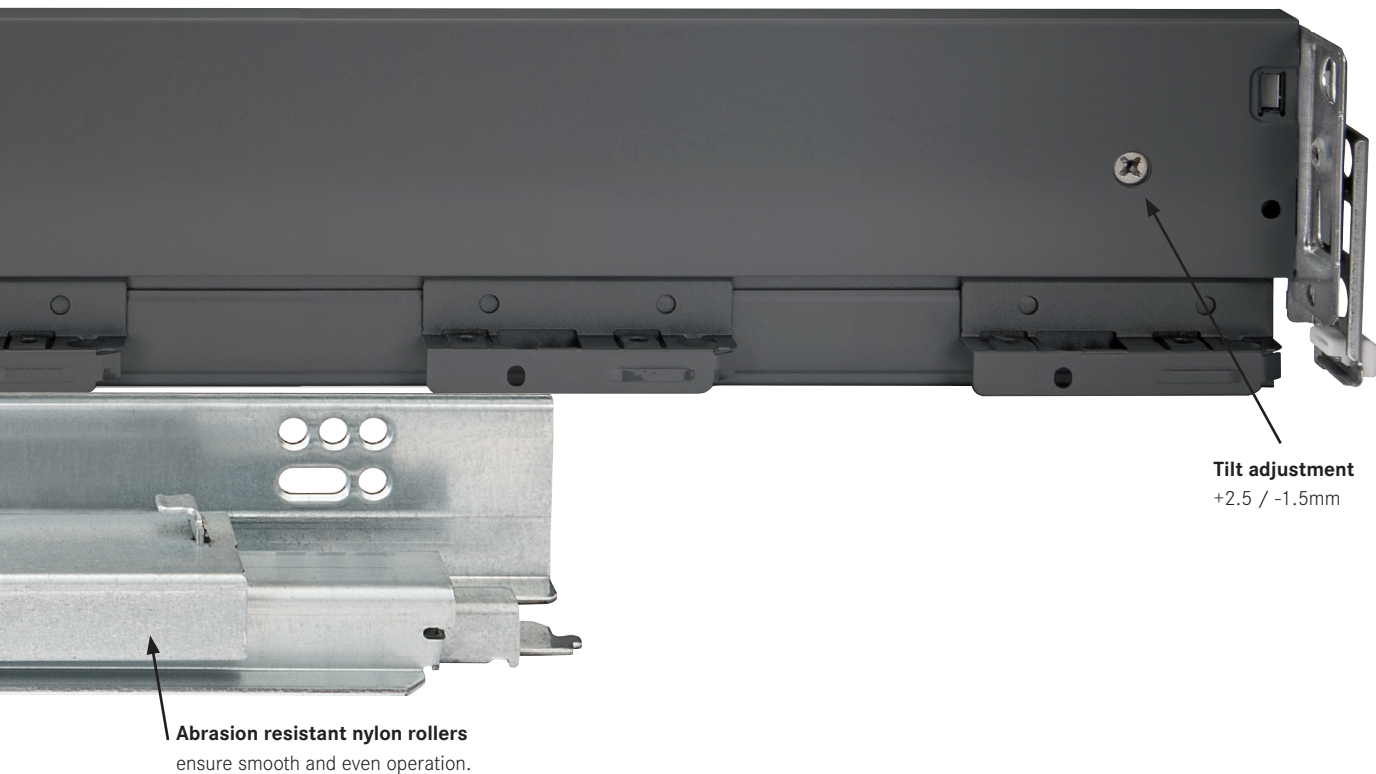
Tipmatic Soft-close for handle-free drawers
