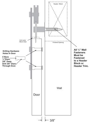
Center Line of Track Mounting Bolts = 1-3/4" + Net Door Height Above Finished Floor
