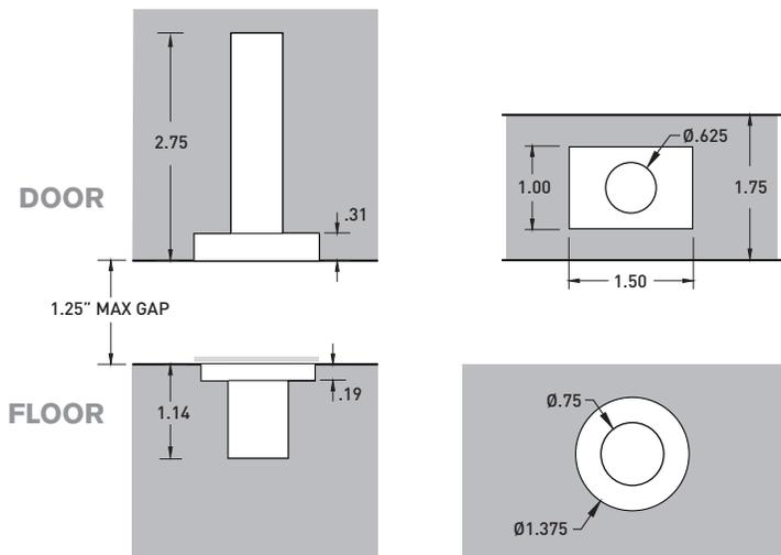
**EXTRA STRIKE SETS**, to create positive stops in both open and closed positions, include the circular strike coverplate, the delrin strike w/ramp, larger magnet, and fasteners. These can be ordered using product code: **GHSTP-300XL-ST-XXX-X**
