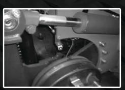
Optional electronic fuel control solenoid can be mounted to LPG powered engines to automatically control top travel speed.
