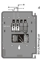
To next agent release initiating device or ELR if last device on circuit
