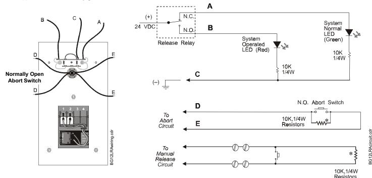
\*Mount End of line resistor on last unit.
